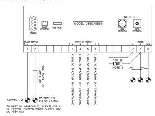
TERMINALS SUITABLE FOR 22-16 AWG (0.6mm² - 1.3mm²) FIELD WIRING TIGHTENING TORQUE = 0.8 Mary (764-4m) b in)
