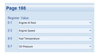
The register address is obtained from the formula: register\_address=page\_number\*256+register\_offset. To read the *Engine Speed* from the above register, the MODBUS master device needs to read the data in two registers and then combine the data from the Most Signficant Bit and the Least Significant Bit. MSB address in Decimal = (166 \* 256) + 2 = 42498 LSB address in Decimal = (166 \* 256) + 3 = 42499
